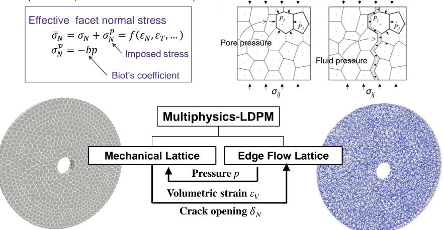
Poroelasticity problem, radial expansion in a thick-walled cylinder due to pore pressure.
