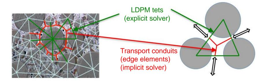
Different meshes for coupled physical fields and mechanical fields!
